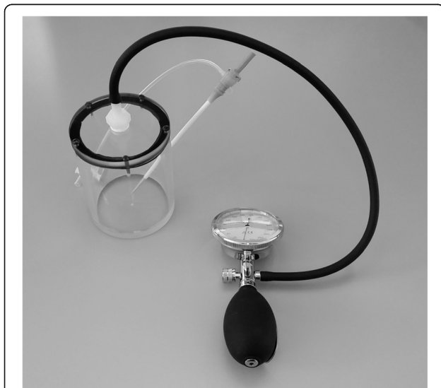
Fig. 1 Structure of the fluid-container phantom. The air-tight container allowed aspiration under different pressures to mimic different common carotid artery-stump-pressures. The pressure in the container was controlled via a sphyngomanometer and was adjusted manually during aspiration
