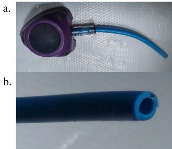
**Fig. 3** Edges of the fractured catheter. **a** The vertical catheter fracture at a point 4 cm from the connector, which was circumferentially aligned. **b** The edges of the fractured catheter were rounded and polished. Upon removal of the TIVAP septum, the cross-section of the fracture was dull, with an overall elliptical shape
