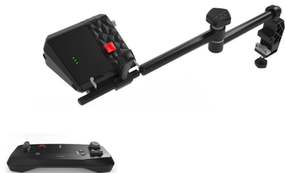
Fig. 1 The liberty bedside robotic drive mounted on the mounting arm, and the hand-held remote-controller
